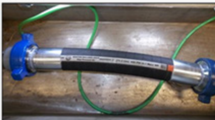
Hose-Union assembly in tester prior to ASTM D380 hydrostatic test
