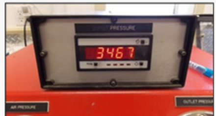
Hose failure at 3467 psi. (exceeding 4:1 safety factor)
