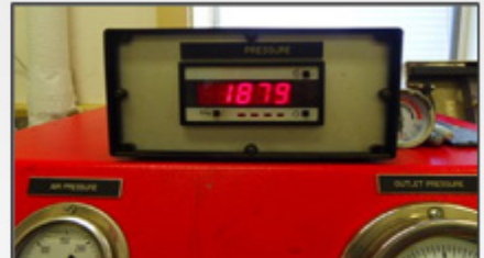
Hose failure at 1879 psi. (exceeding 4:1 safety factor)
