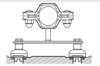
Bracket's cups/boots mount flush to IMP, encasing rivet nuts while silicone rubber gasket create a seal to surface
